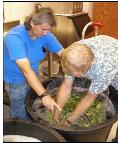
Figure 6. Cylindrical mesh basket in wash drum.
